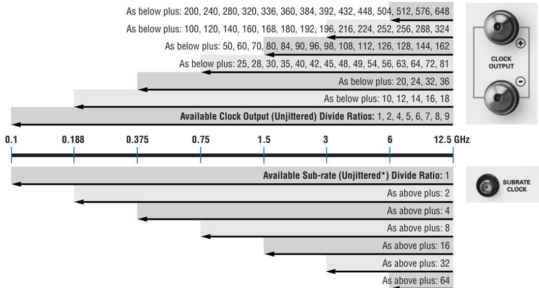
\* This output can also provide a full-rate jittered clock.
