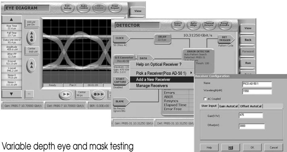
An external optical receiver may be added to the input of the BERTScope detector. Through the user interface it is easy to input and save the characteristics of the receiver. Once accomplished, relevant units on physical layer displays are changed to optical power in dBm,  $\mu$ W or mW. Coupling may be AC or DC, and the software steps the user through dark calibration.
