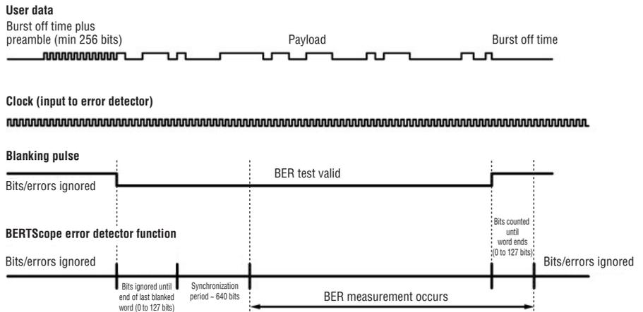
BERTScope word size is 128 bits. An example timing diagram is shown here for a PRBS payload. Counting of bits will not start until a 128 bit word boundary occurs, meaning that after the blanking pulse transitions, up to 127 bits may pass before synchronization begins. For a PRBS, synchronization typically takes 5 words, or 640 bits. Similarly, bit measurement will continue for up to 127 bits after the blanking signal transitions again. RAM-based patterns take longer to synchronize.
