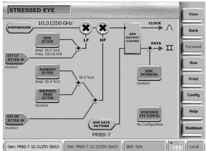
**Notes:** Specified for data rates from 1.45 Gb/s to 11.2 Gb/s. Usable with limited performance to 622 Mb/s. Internal RJ, BUJ, and external high frequency jitter input limited to 0.5 UI, combined. Rear panel low frequency jitter input can be used to impose additional jitter; SJ and external jitter sum total cannot exceed jitter magnitude limits given for SJ below.
