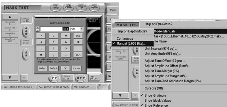
For eye diagrams and mask testing, the depth of test may be varied in manual mode; the instrument will take the specified number of waveforms then stop. The range is 2,000 to 1,000,000 bits (complete waveforms). Alternatively, the default mode is Continuous, and the eye or mask test increases in depth over time.
