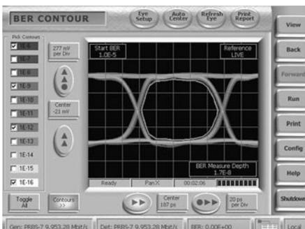
The live data option is designed to measure parametric performance of traffic that is either unknown or non-repeating. This can include traffic with idle bits inserted such as in systems with clock rate matching. It is also suitable for probing line cards, etc.
